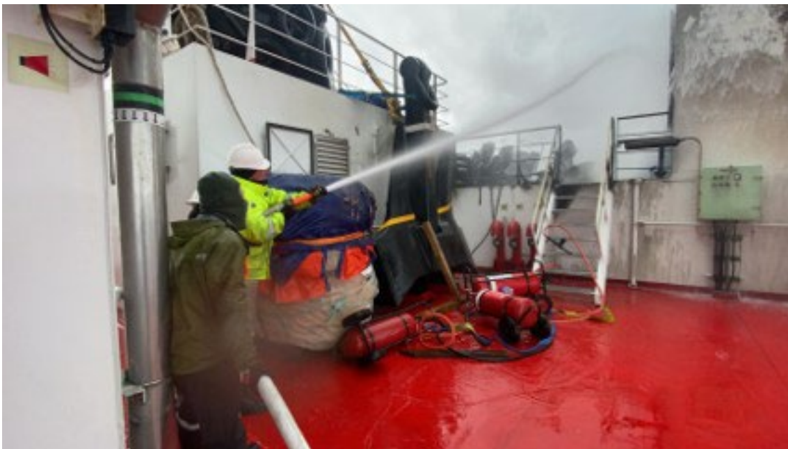
Figure 5: Boundary cooling and firefighting operations on deck
