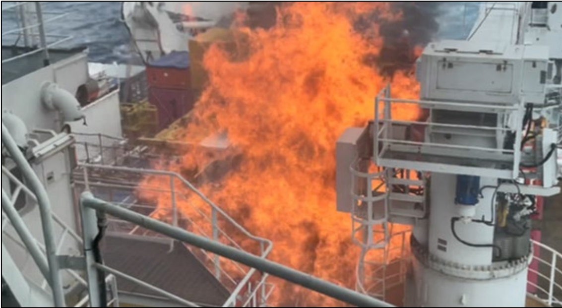
Figure 4: Flames from the port engine room exhaust ventilation casing
