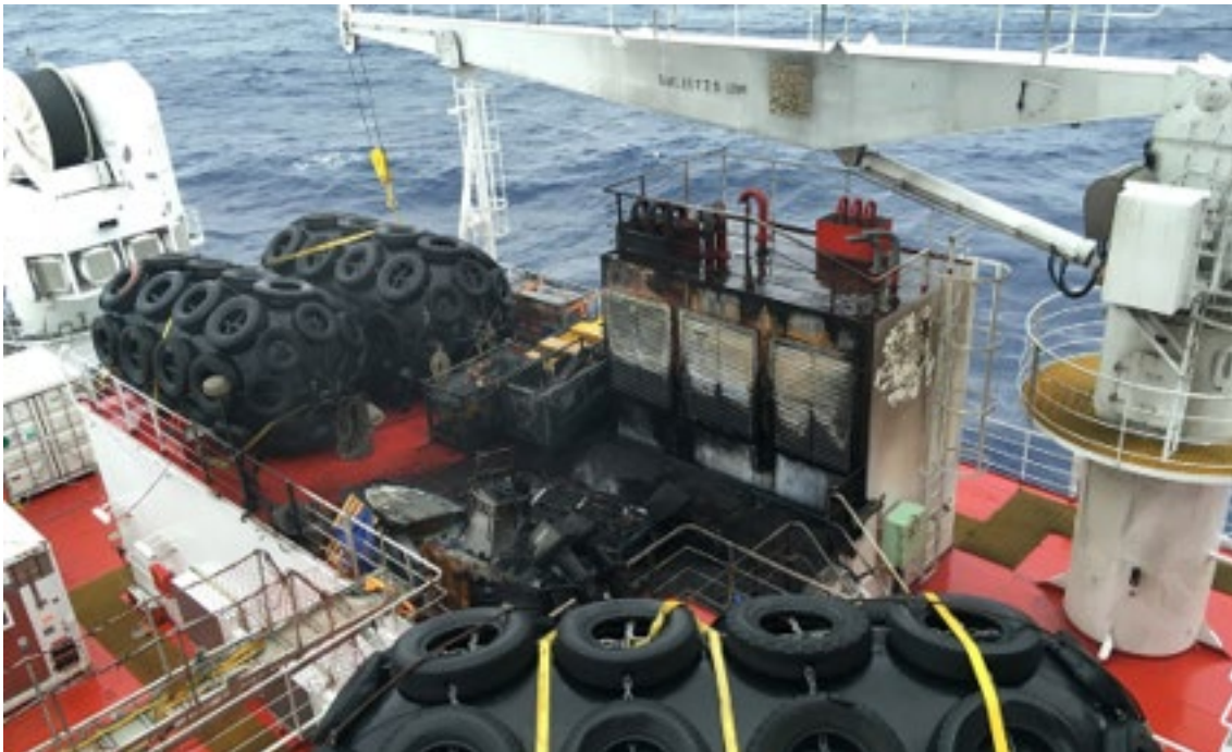
Figure 7: Fire damage on deck including the burnt-out watercraft adjacent to the casing
