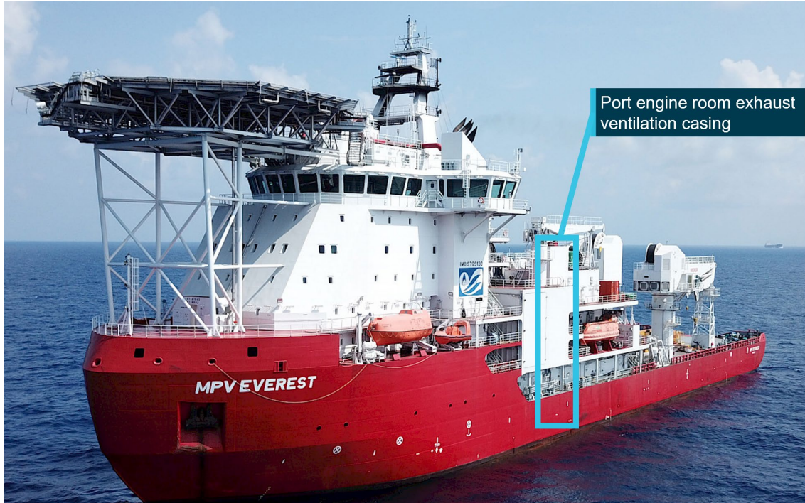
Figure 3: MPV Everest – Port engine room exhaust ventilation casing
