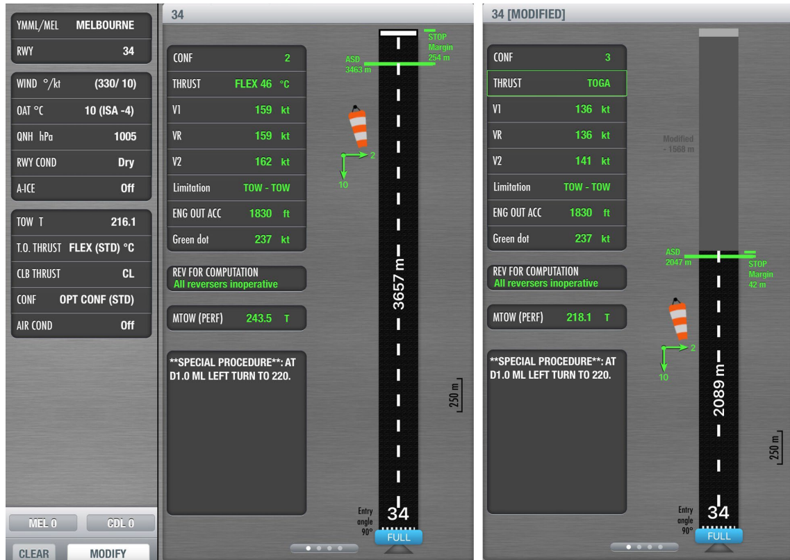
Figure 5: 9M-MTL Airbus Flysmart performance comparison between Melbourne runway 34 full-length (centre of image) and reduced-length (right) under otherwise identical conditions.
