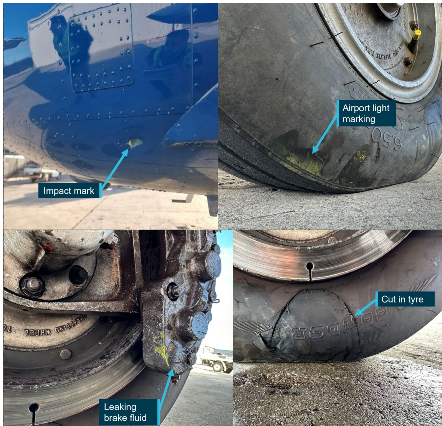
Figure 3: Damaged sustained by VH-XMM
