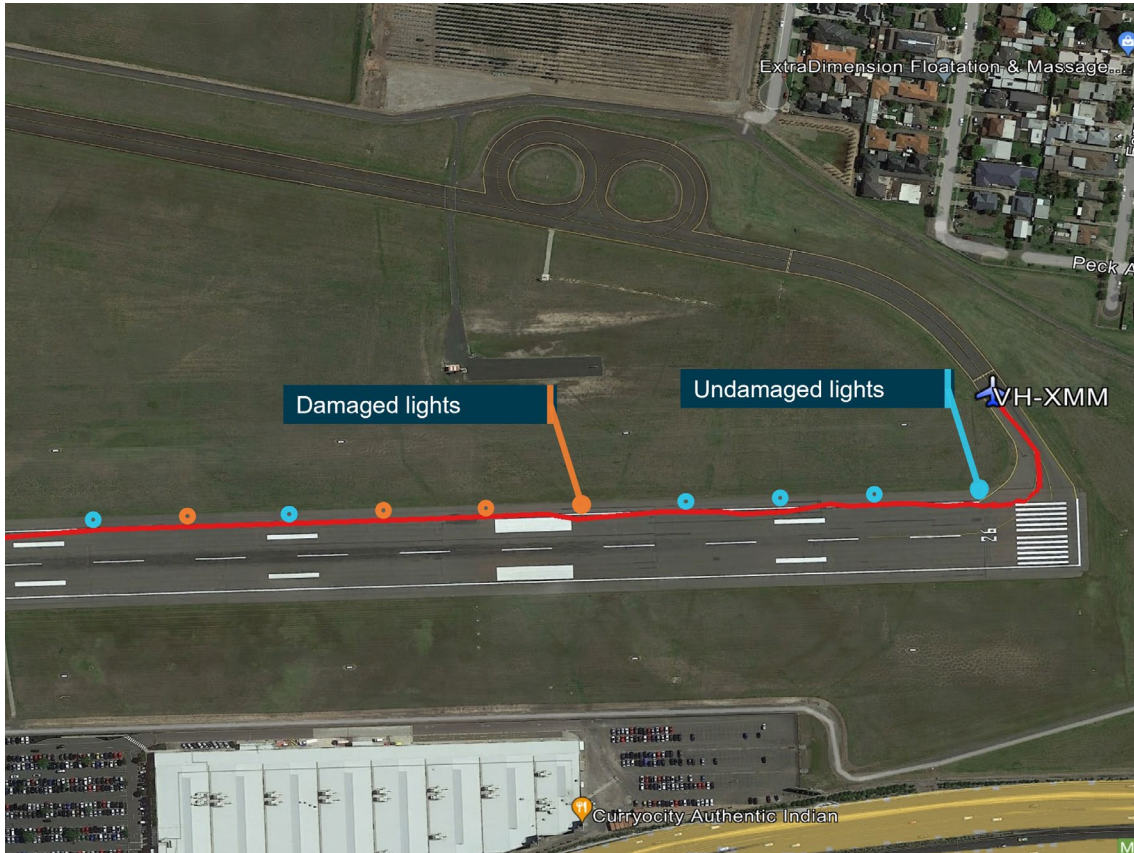
Figure 5: VH-XMM take-off path with damaged light positions
