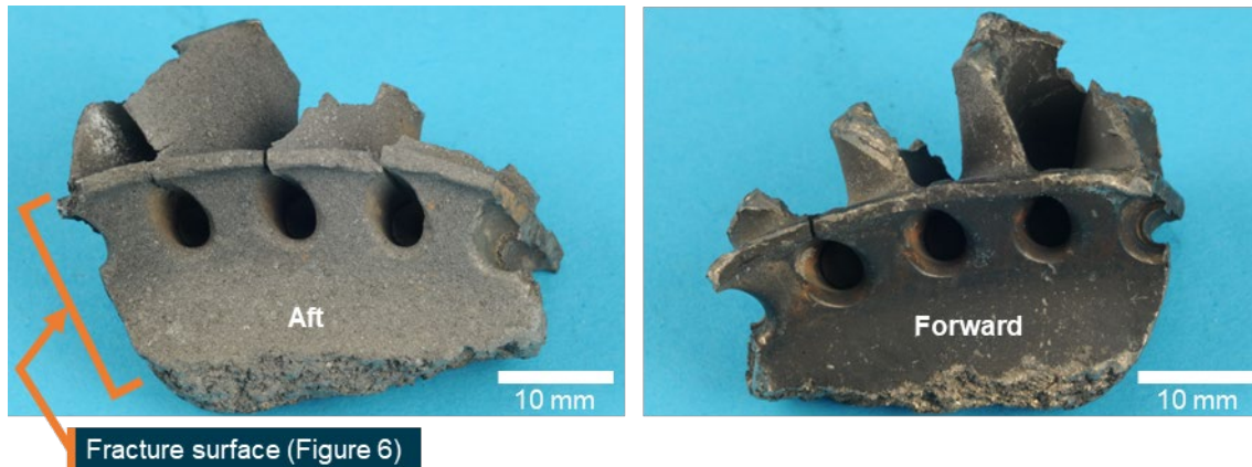
Figure 5: Recovered fragment of 3rd-stage turbine wheel found lodged in the combustion case viewed from the aft (left) and forward sides (right)
