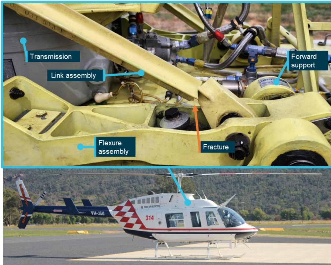
Figure 1: Right, forward, pylon support link assembly fracture
