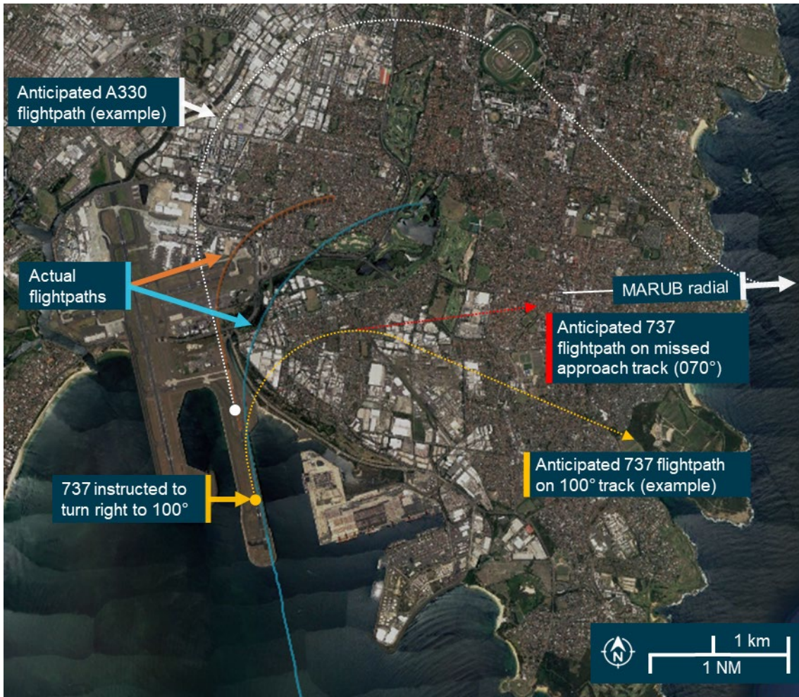
Figure 16: Trainee ADC’s likely mental model of the approximate flight paths the aircraft were expected to take after issuing the instruction for the 737 to turn
