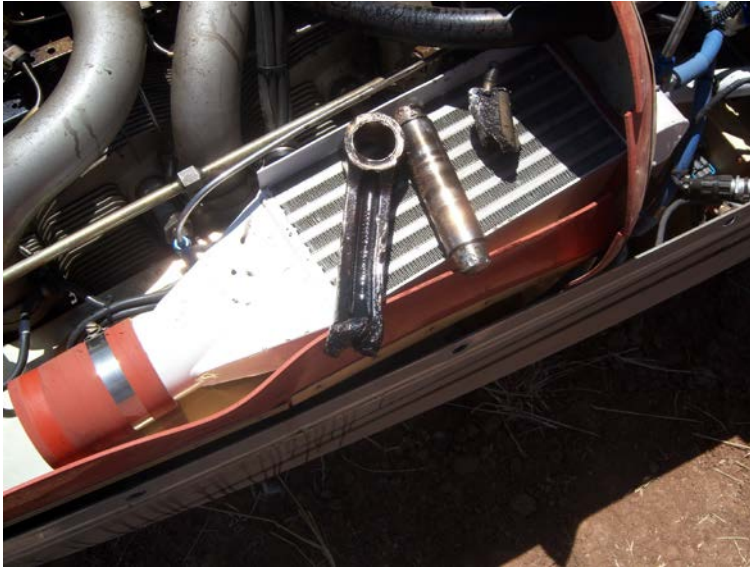
Figure 3: Engine number two cylinder failed parts
