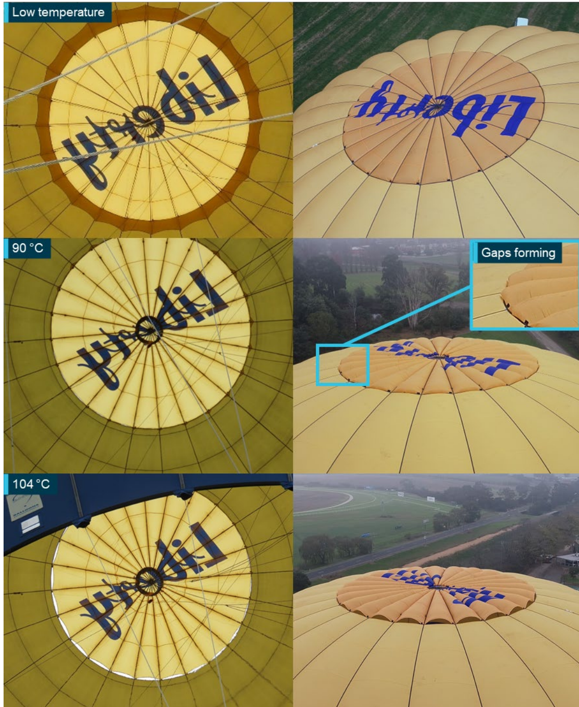
Figure 9: Deflation system testing
