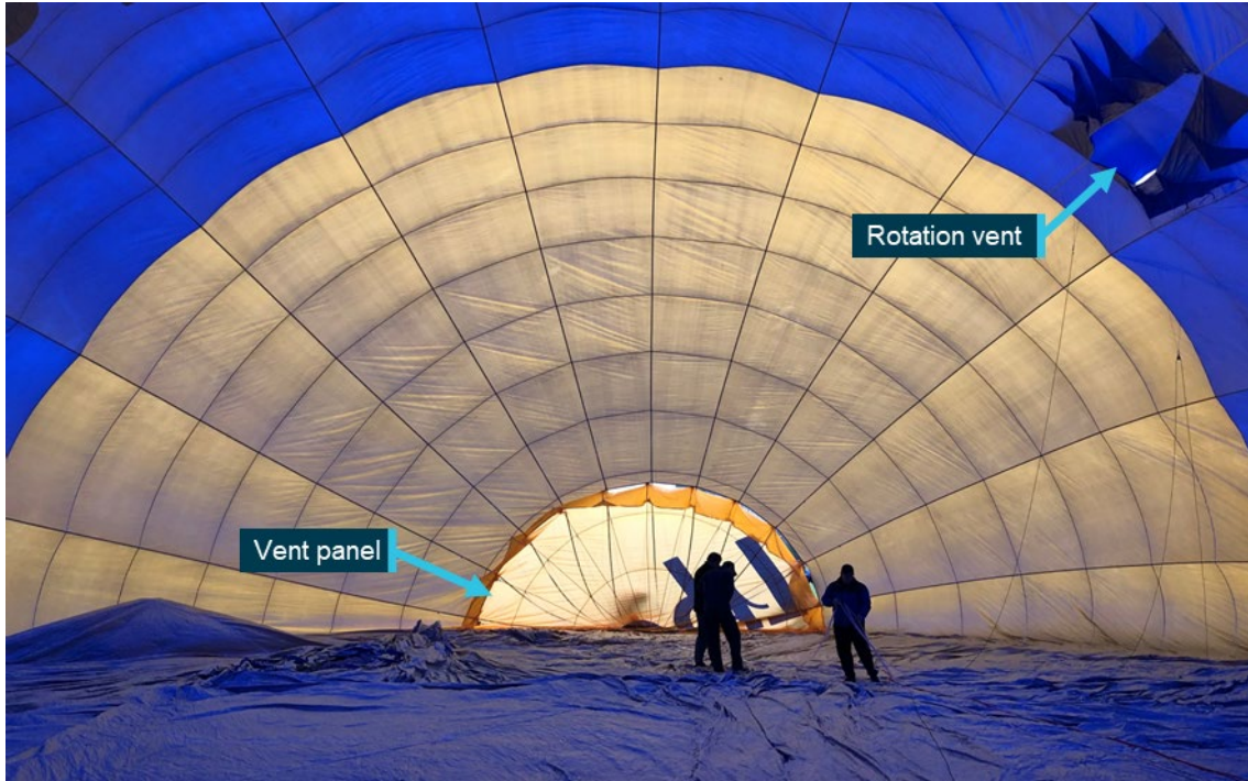
Figure 8: Internal envelope inspection
