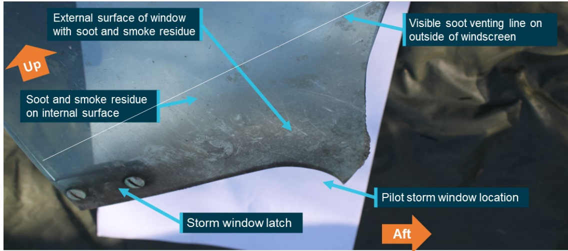
Figure 9: Smoke and soot indications on window surfaces adjoining the pilots storm window
