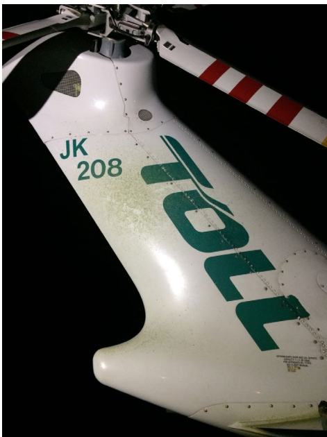
Figure 4: Evidence of foliage contact on the vertical fin
