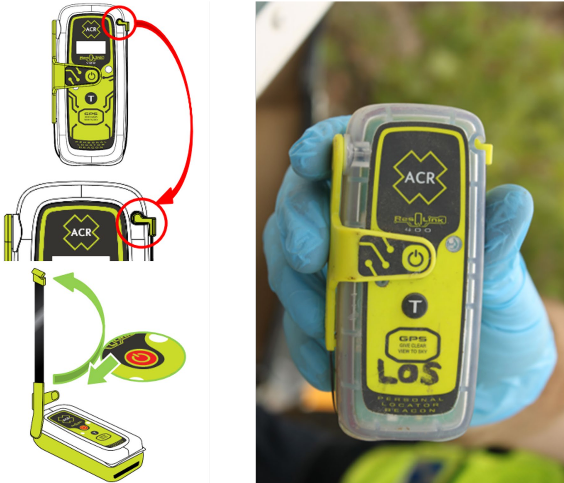
Figure 4: ResQLink activation instructions (left) and condition in-situ at VH-LOS accident site (right). The image on the right shows the antenna and power button guard remained in the down position
