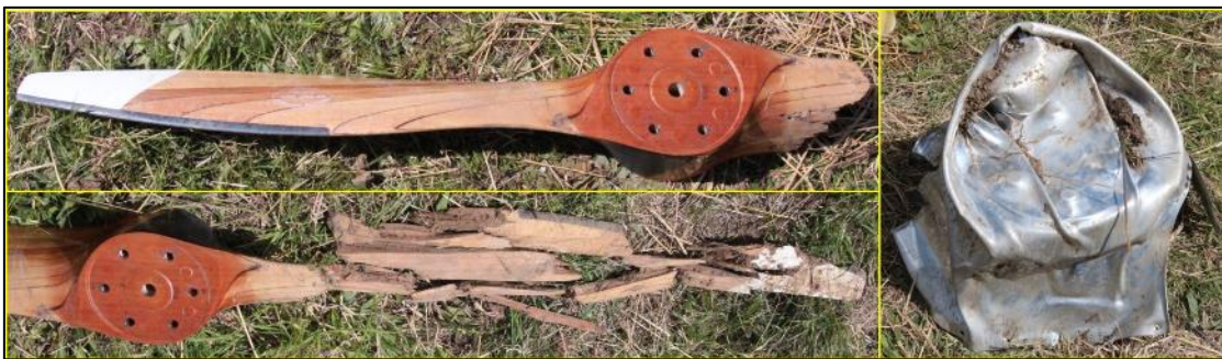
Figure 3: Broken two-bladed propeller blade and metal spinner, showing the reconstructed detached/shattered blade
