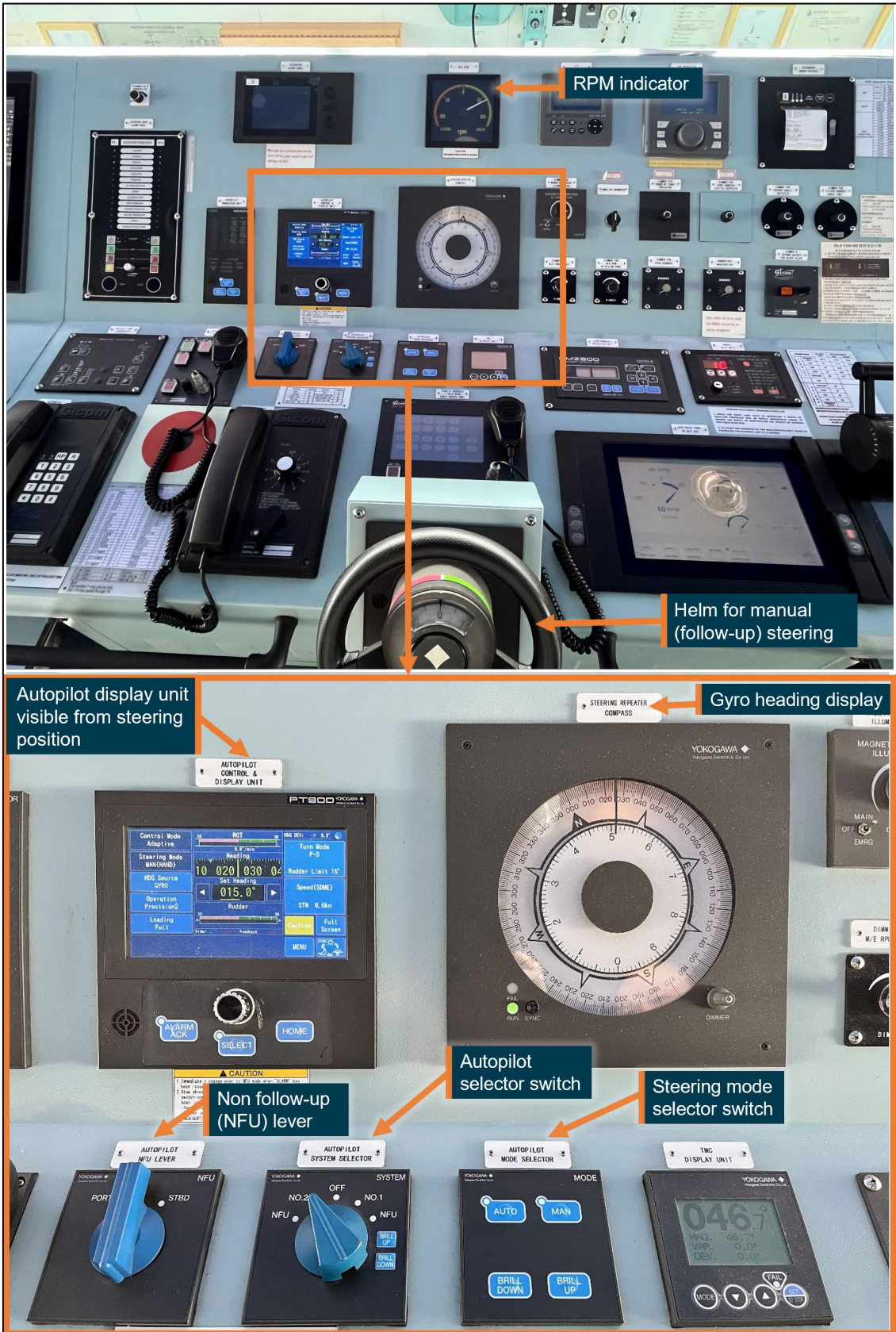
Figure 5: Hagen Oldendorff's bridge console layout showing the control and display unit
