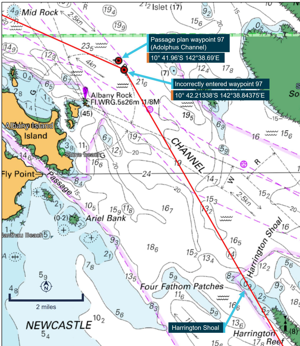
Figure 9: Section of chart Aus 839 showing incorrectly input waypoint
