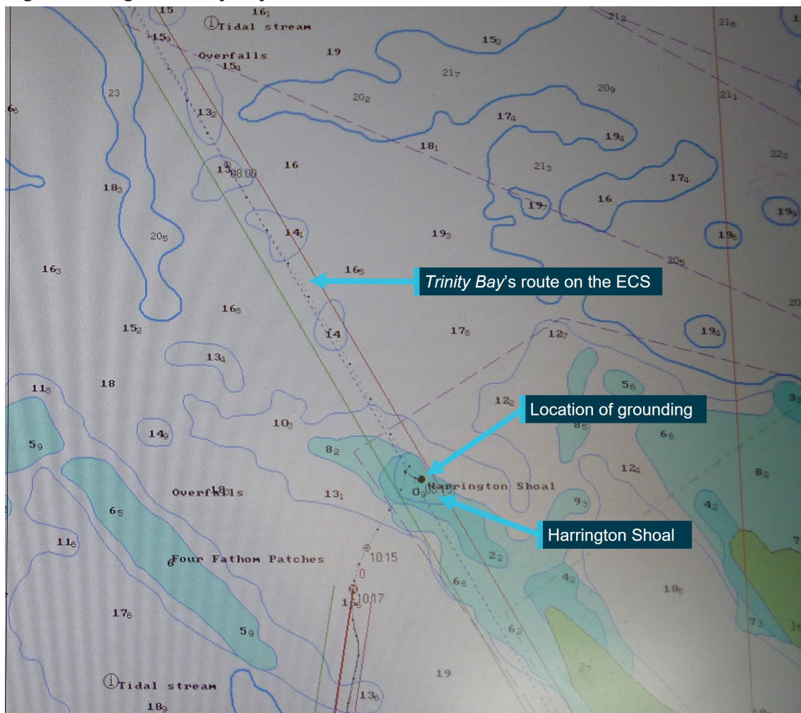
Image of TRANSAS ECS screen taken after grounding showing Trinity Bay's planned route and track in vicinity of Harrington Shoal. Source: Sea Swift, annotated by the ATSB.
