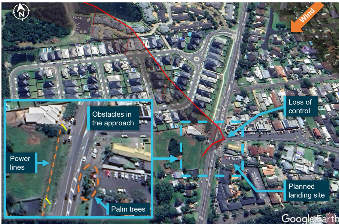
The flight track extracted from the helicopter GPS is shown in red. The inset shows the proximity of the obstacles (power lines and palm trees) under the approach to the planned landing area. The relative wind can be seen to be almost perpendicular to the track from the left, an area of known hazard for the onset of LTE.
