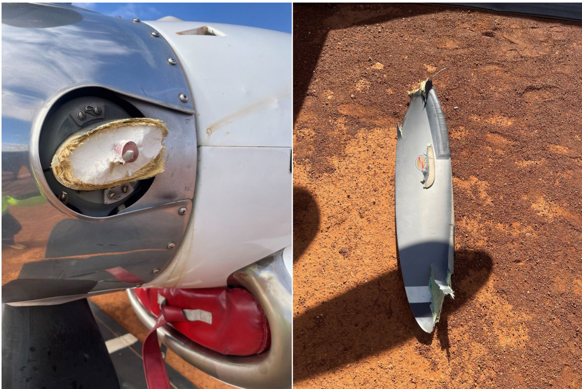
Figure 3: Propeller hub and detached propeller
