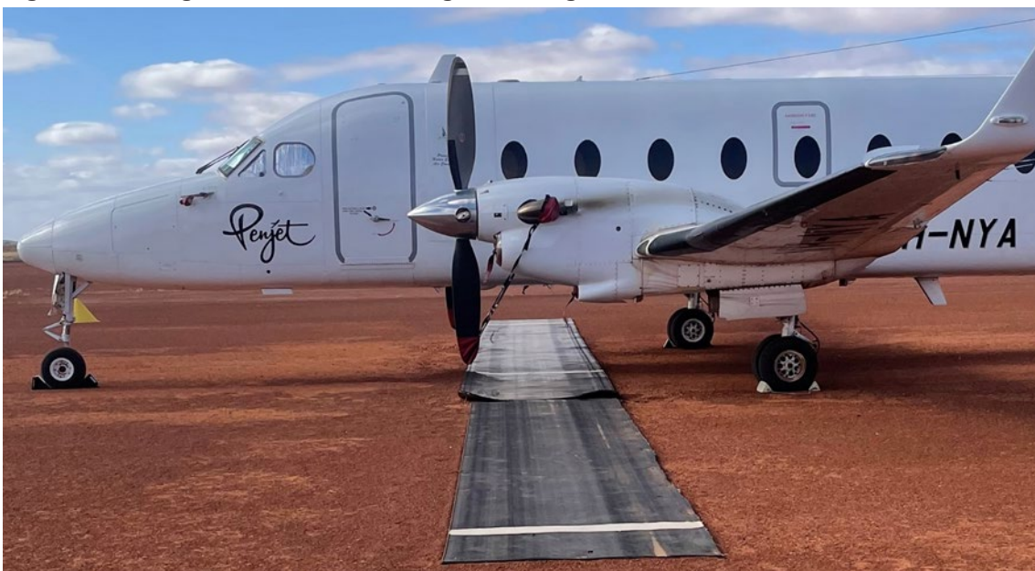
Figure 1: Damaged aircraft and dislodged matting
