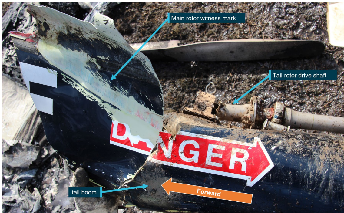
Figure 4: Tail boom impact
