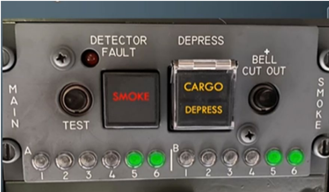
Figure 1: Main deck cargo smoke detector panel
