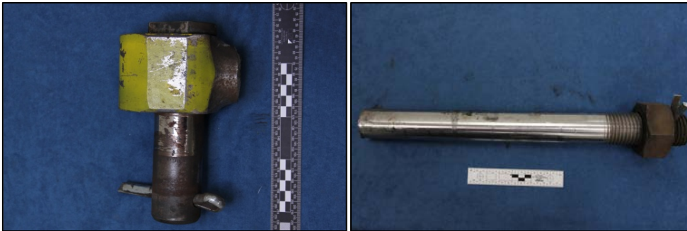
Figure 14: Fractured segments of drawbar tail pin
