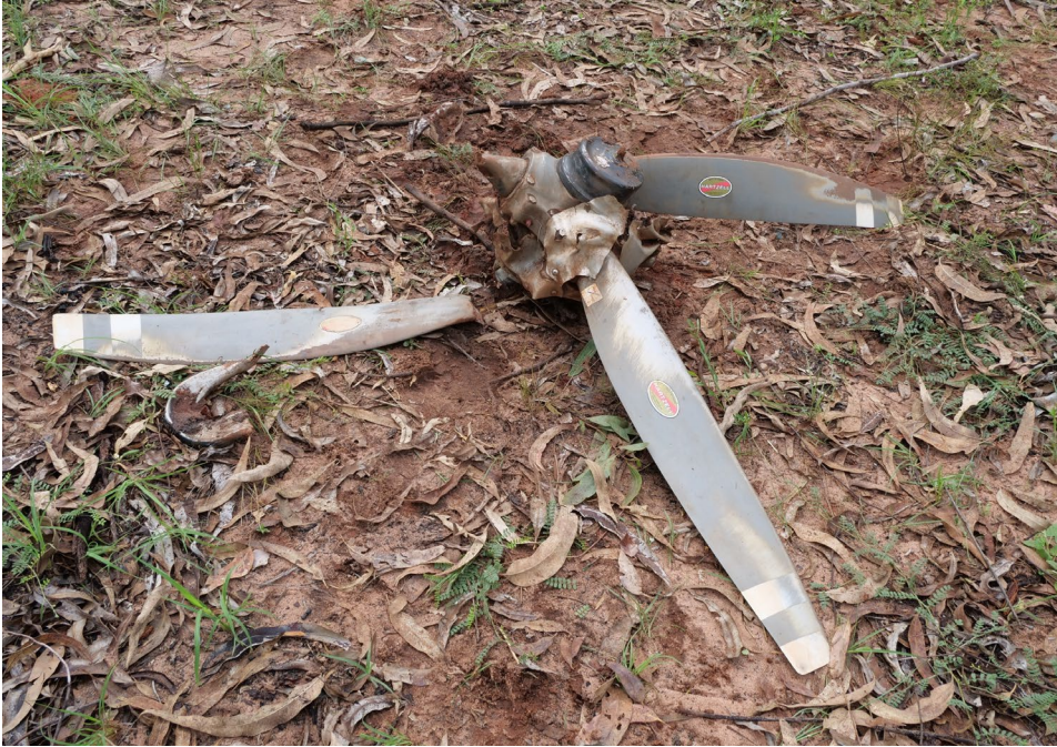
Figure 6: Propeller assembly as removed from the ground impact crater
