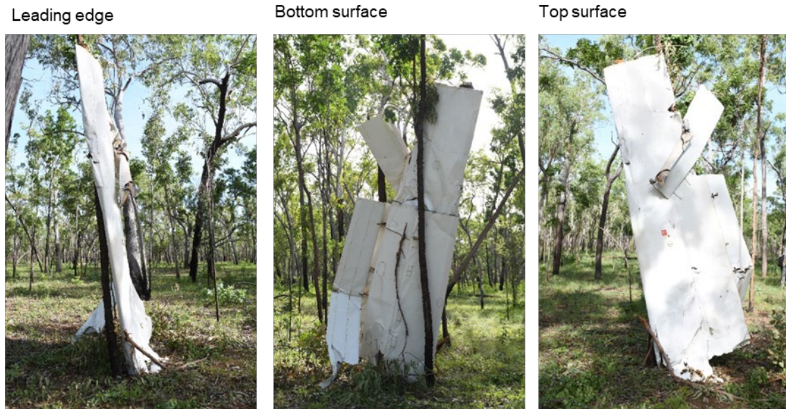
Figure 3: As found position of the right wing approximately 300m from the main wreckage
