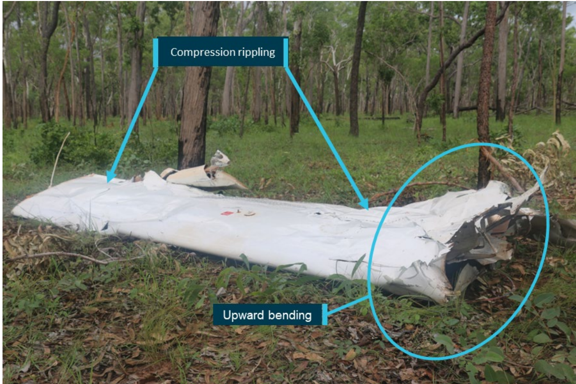
Figure 5: Separated right wing assembly showing damage associated with significant upward bending forces
