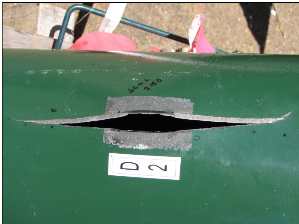
Figure A7: Flaw D2, after testing – failure by bursting (rupture)
