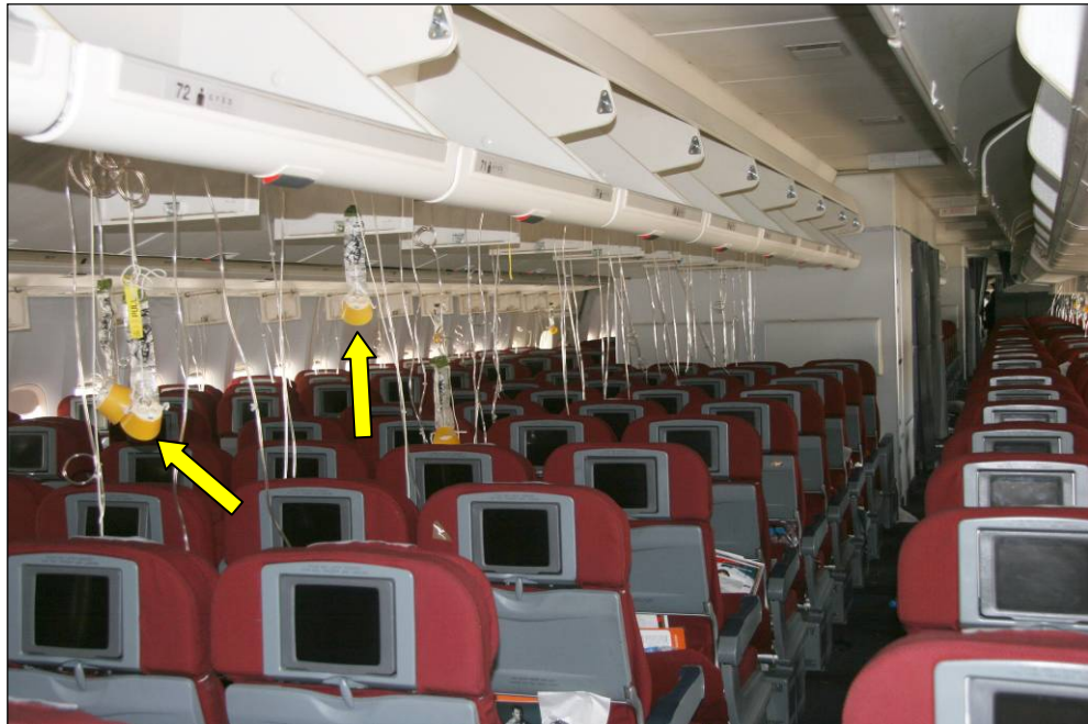
Figure 26: Typical appearance of the cabin after arrival in Manila. Note the passenger masks dropped and activated, and those dropped and not activated (arrowed)
