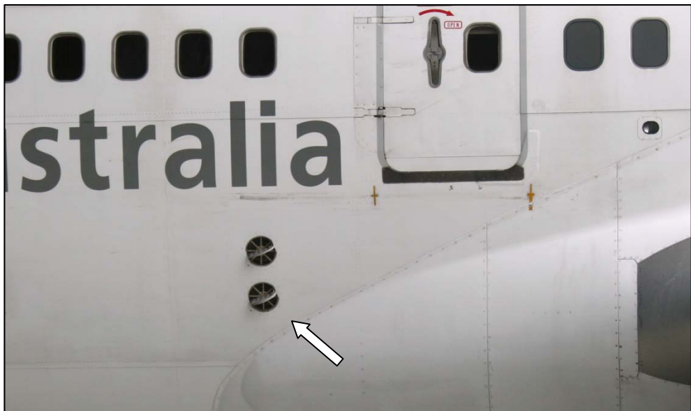
Figure 8: Pressure relief valve blowout doors open (arrowed)
