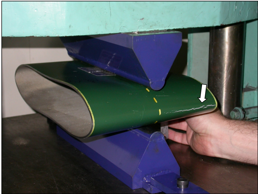
Figure 61: Completed flattening test, with area of cracking arrowed
