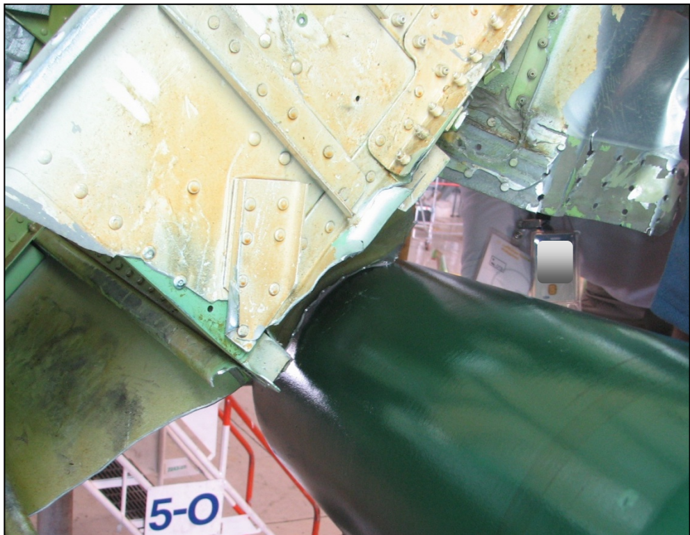
Figure 6: Oxygen cylinder held against skin fold to illustrate conformance
