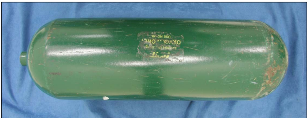
Figure 45: Cylinder S/N 535691 – relatively poor external surface condition
