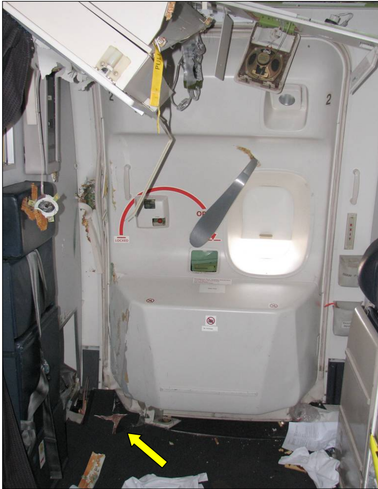
Figure 19: Hole in cabin floor – viewed from position of number-4 oxygen cylinder. Broken yellow lines mark the normal route of the first officer's aileron control cables
