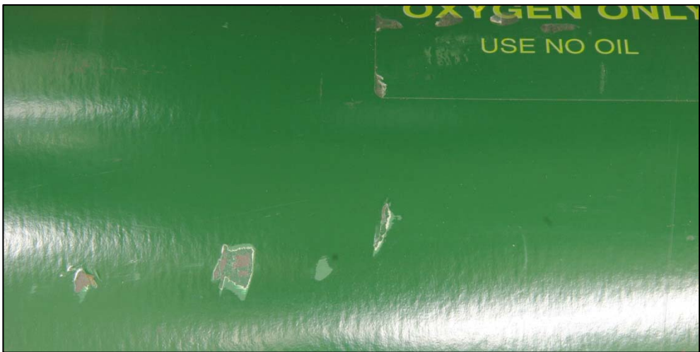
Figure 45: Cylinder S/N 535691 – relatively poor external surface condition
