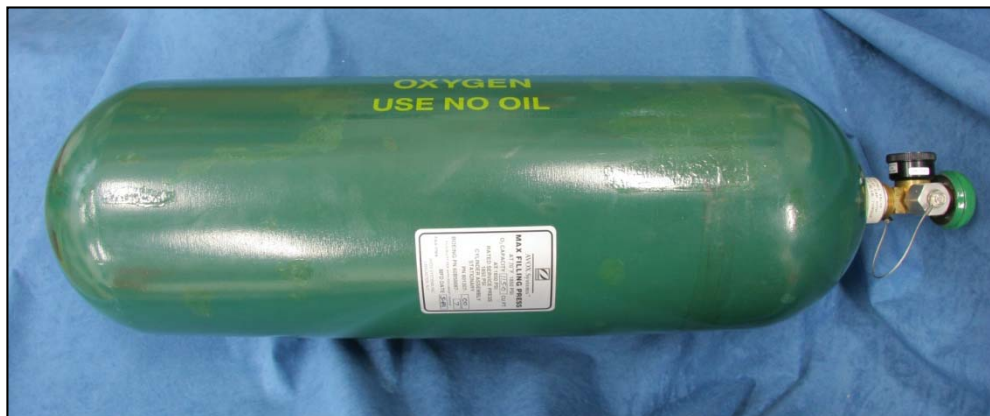
Figure 42: Cylinder S/N 883198 showing typical external condition and labelling
