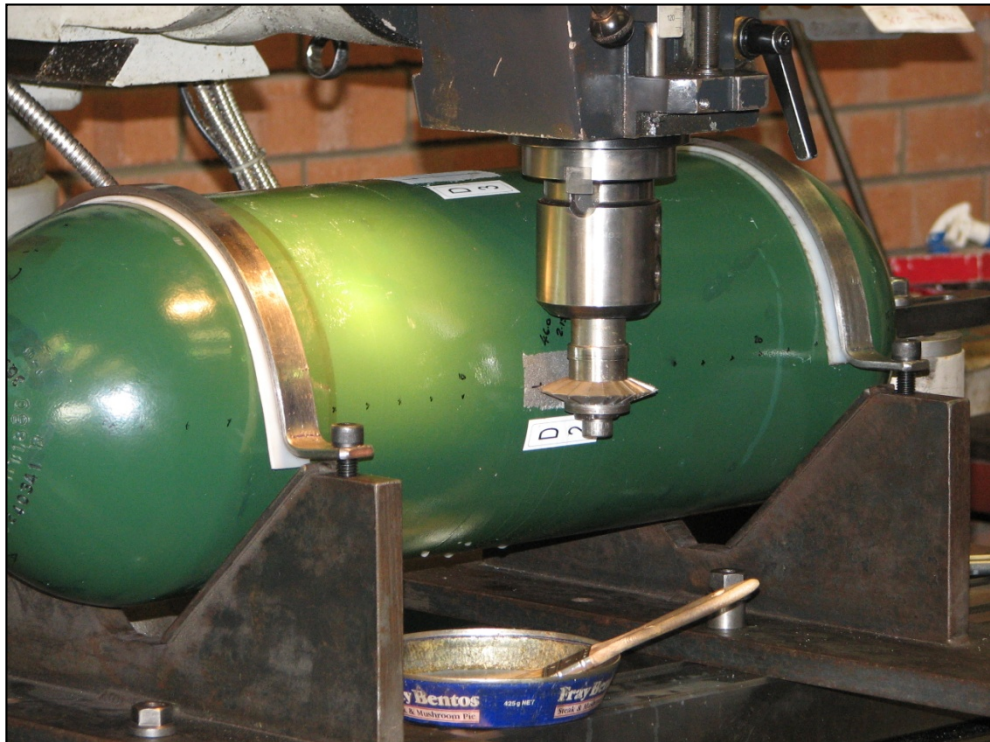
Figure A3: Artificial flaw milling arrangements
