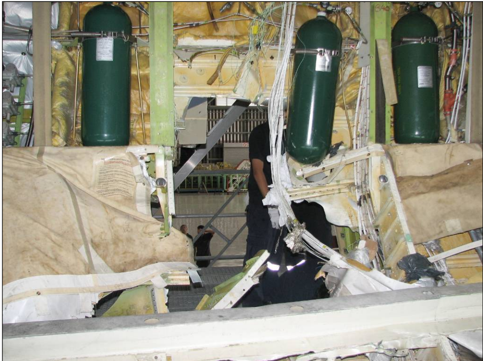
Figure 11: Number-5 oxygen cylinder adjacent to fractured fittings and lines from the number-4 cylinder
