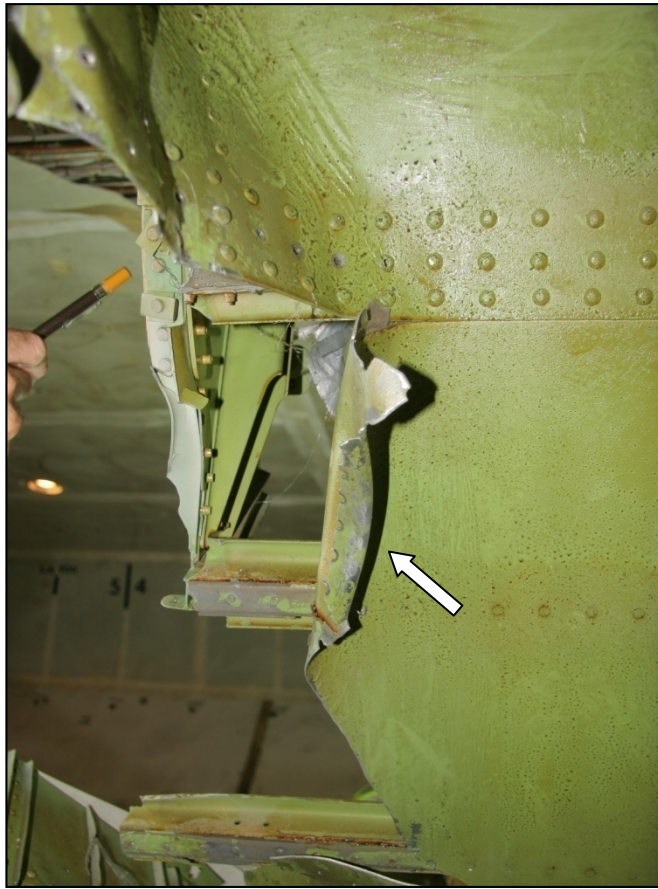
Figure 6: Oxygen cylinder held against skin fold to illustrate conformance
