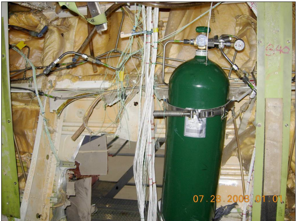
Figure 11: Number-5 oxygen cylinder adjacent to fractured fittings and lines from the number-4 cylinder
