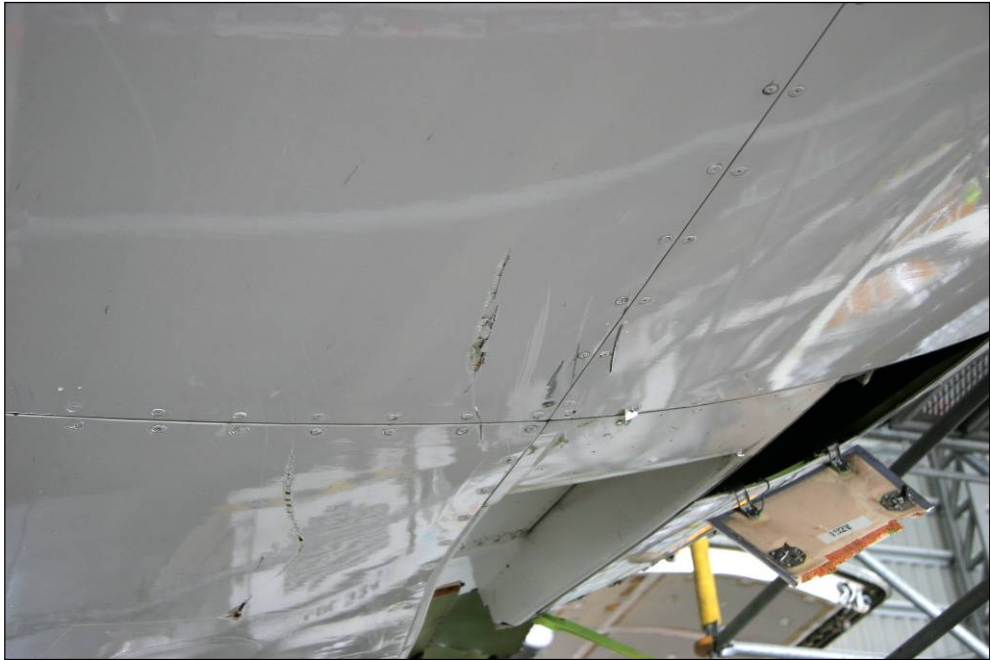
Figure 8: Pressure relief valve blowout doors open (arrowed)
