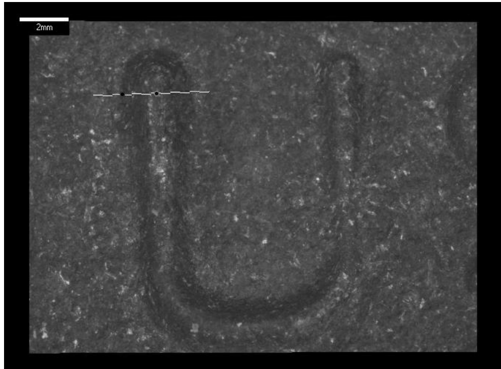
Figure 58: Cylinder stamp marking (letter 'U') with plane of profile measurement shown
