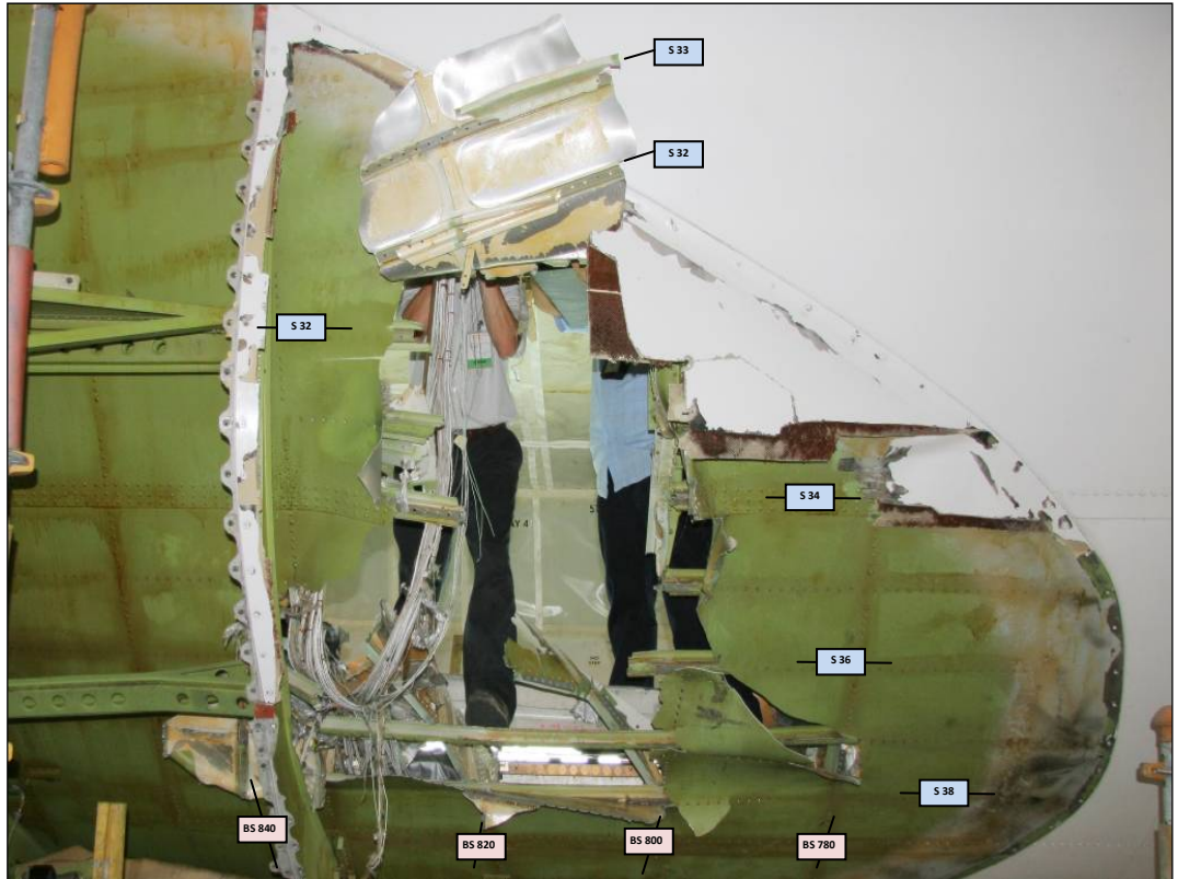
Figure 4: 747-400 forward fuselage Section and Station diagram
