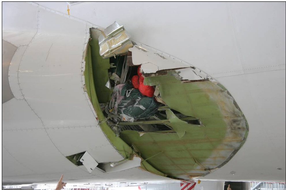
Figure 2: Fuselage rupture with protruding cargo
