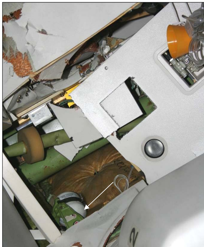
Figure 22: Damage above R2 door, exposing the EPAS cylinder (arrowed)
