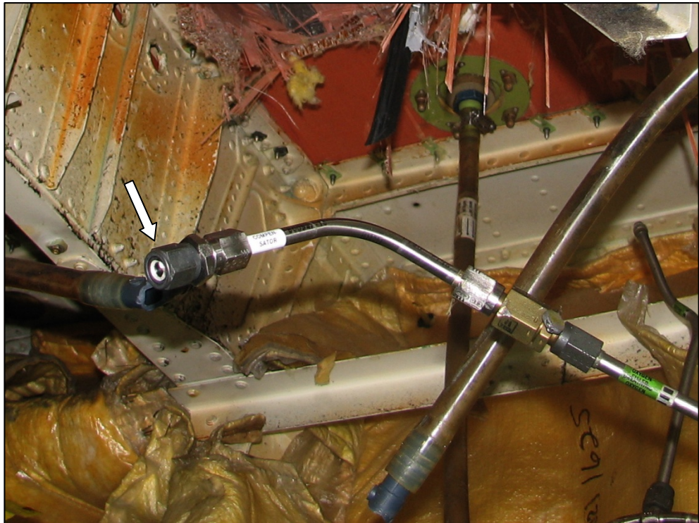
Figure 15: Number-4 cylinder overpressure discharge line fracture (arrowed)
