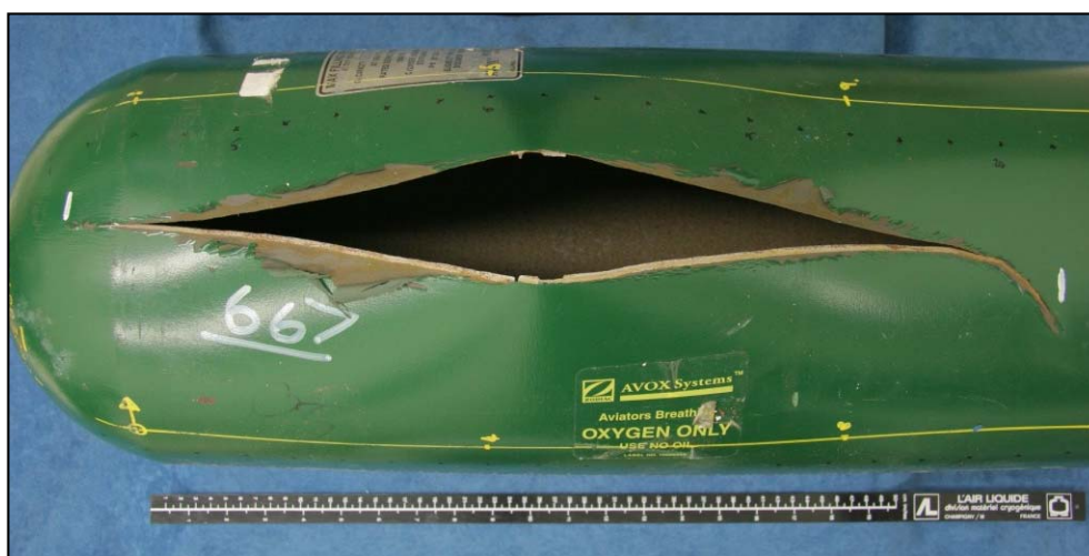
Figure 62: Rupture of cylinder S/N 535667
