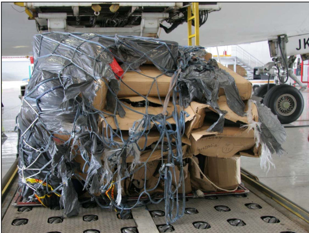
Figure 29: Cargo pallet after removal from the aircraft, showing the end facing the rupture
