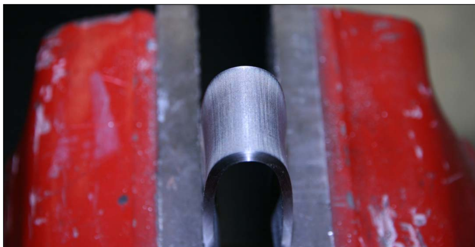
Figure B10: A-Gasol ® sample during bend testing
