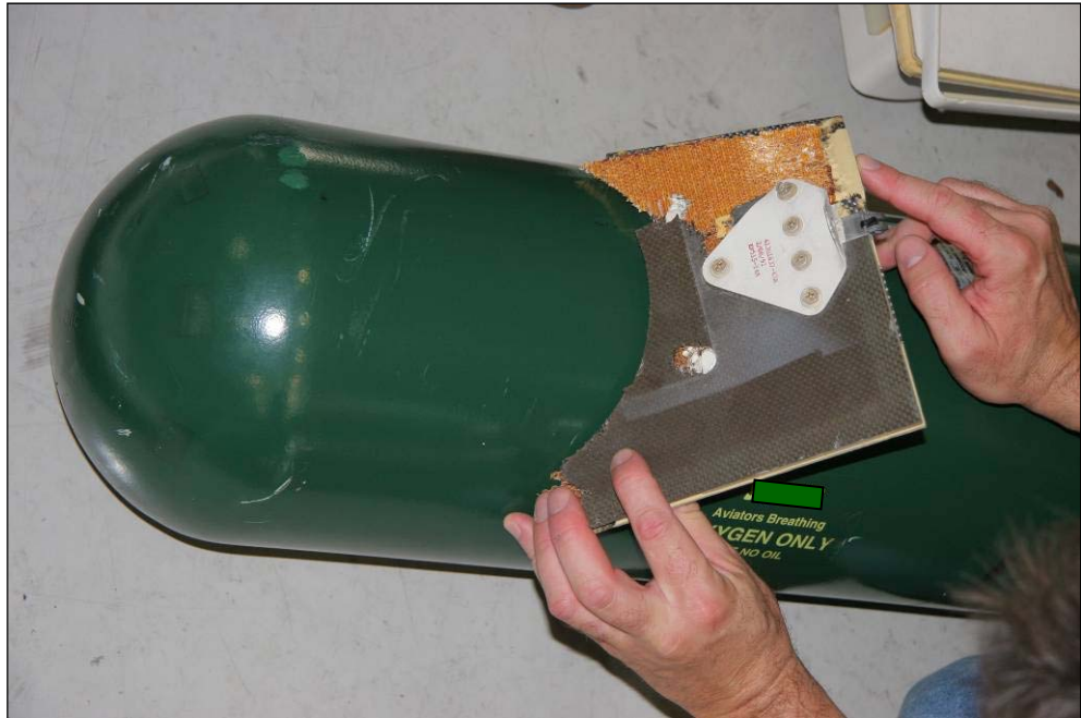
Figure 25: Panel with cut-out placed against another oxygen cylinder to illustrate the conformance in diameter
