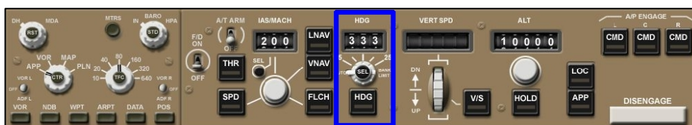
Figure 38: Mode Control Panel (MCP) with the HDG SEL area highlighted
