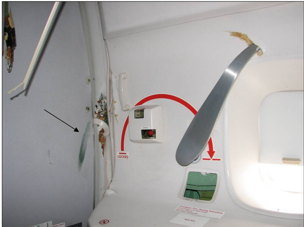
Figure 20: Door frame damage, green paint smear and rotated R2 door handle
