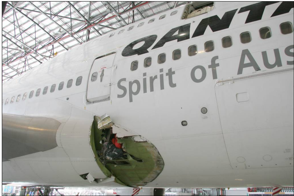
Figure 1: Fuselage rupture – external view
