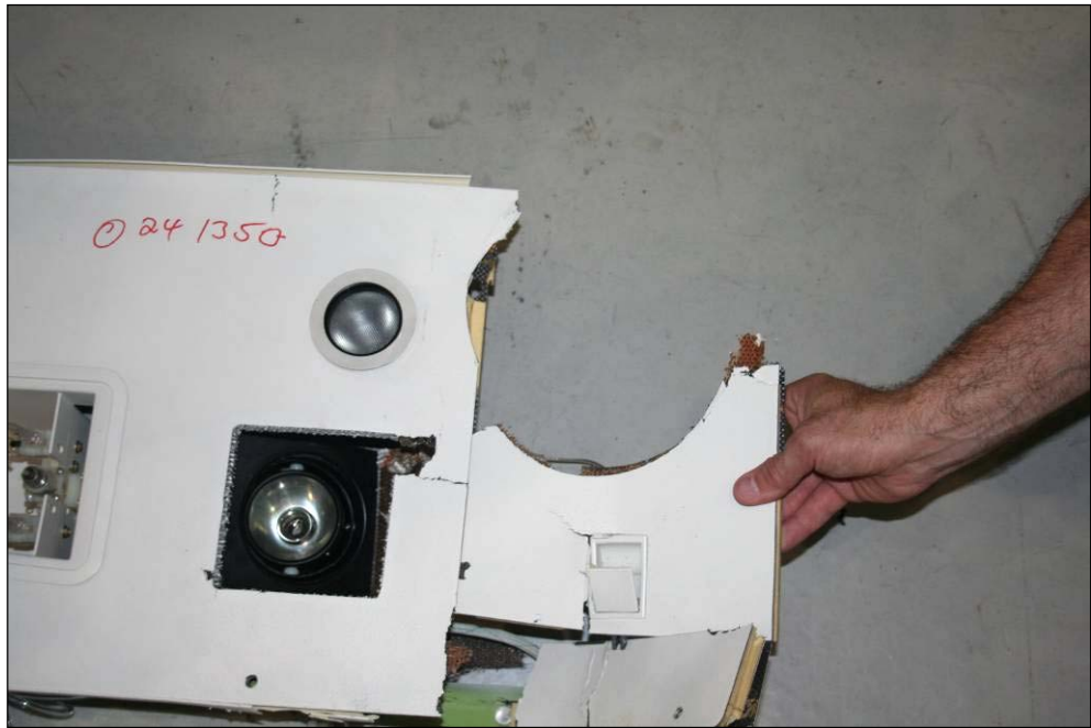
Figure 23: Panels above the R2 door showing circular cut-out area
