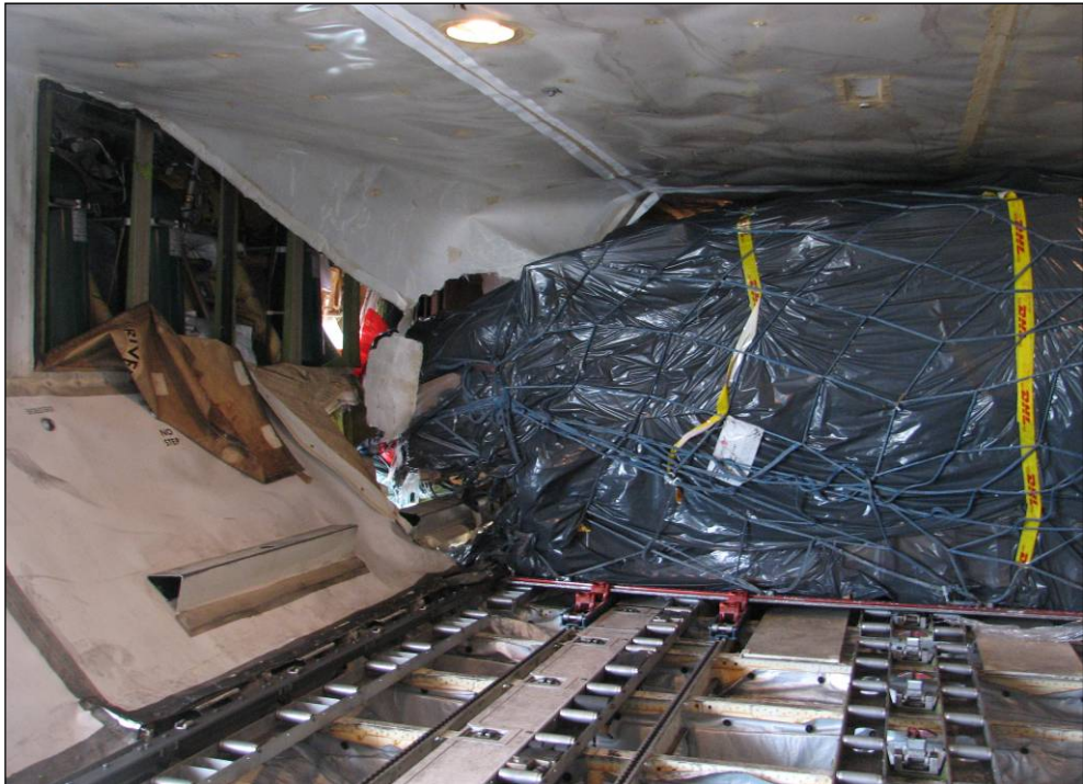
Figure 28: Cargo pallet adjacent to the fuselage rupture (view looking towards the rear of the aircraft)
