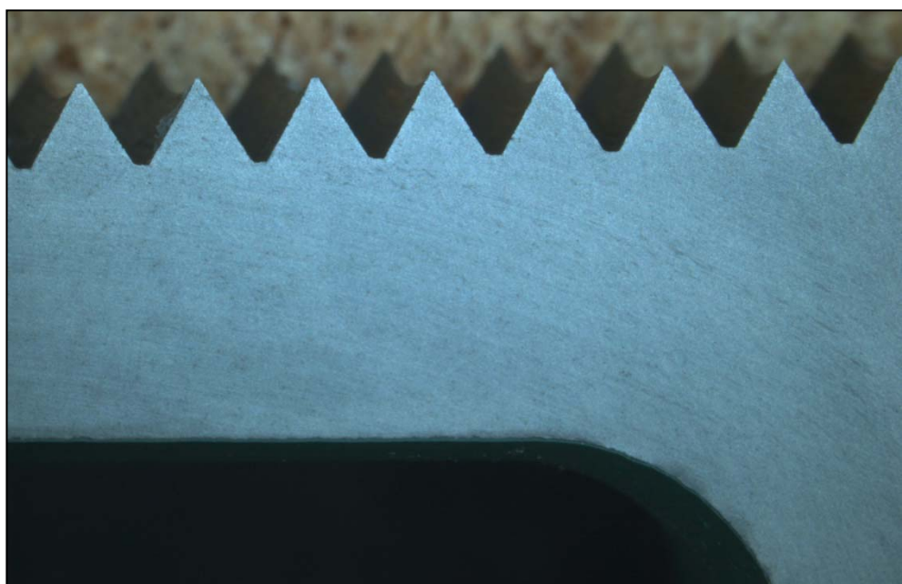
Figure 59: Cylinder neck thread profile
