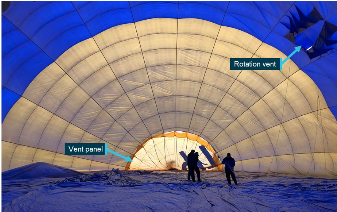
Figure 7: Internal envelope inspection
