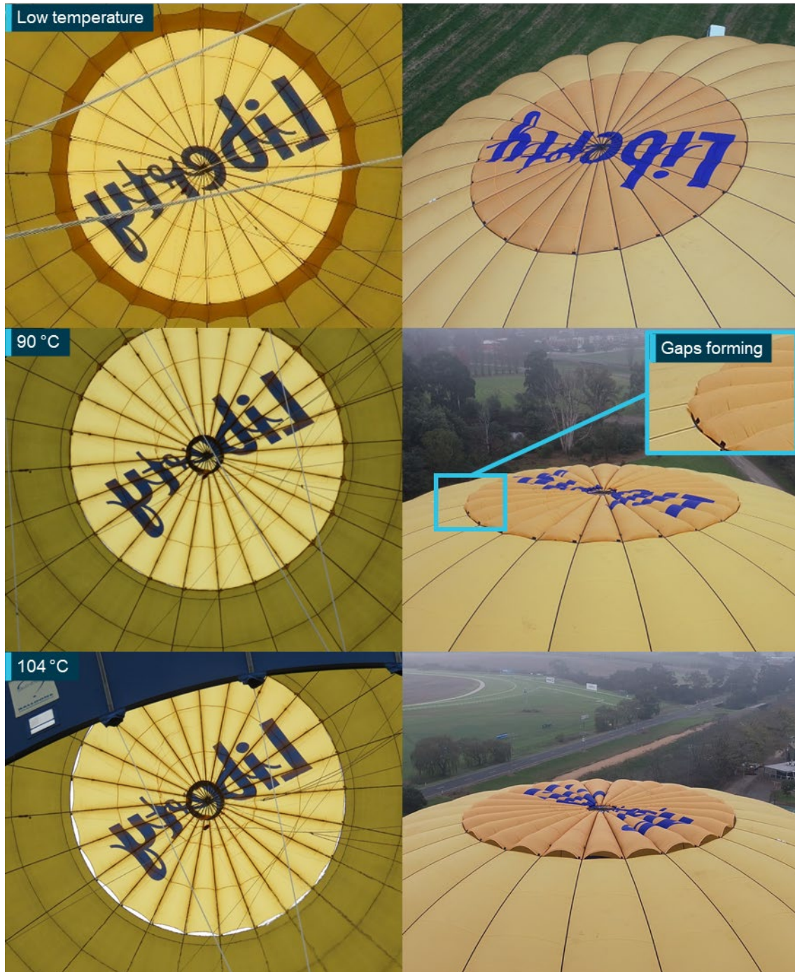
Figure 8: Deflation system testing
