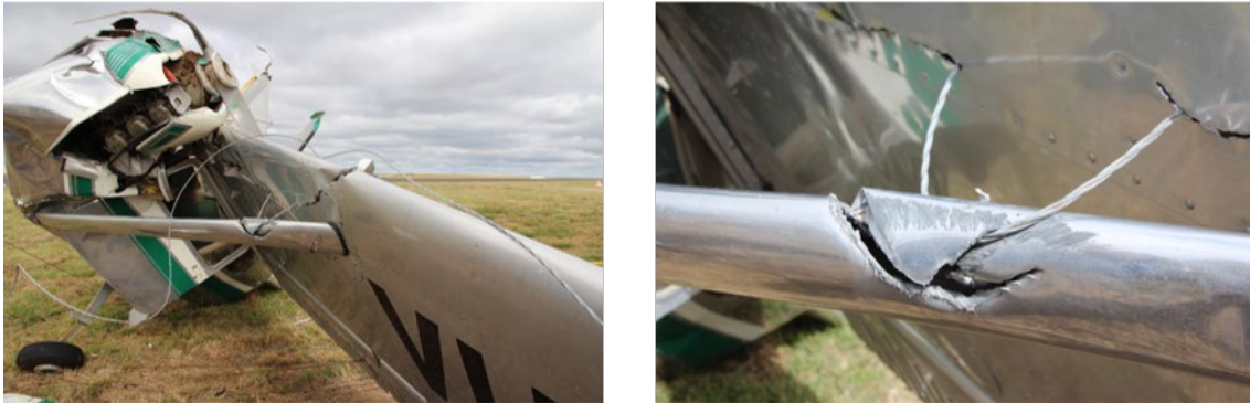
Figure 5: Powerline, left wing and strut
