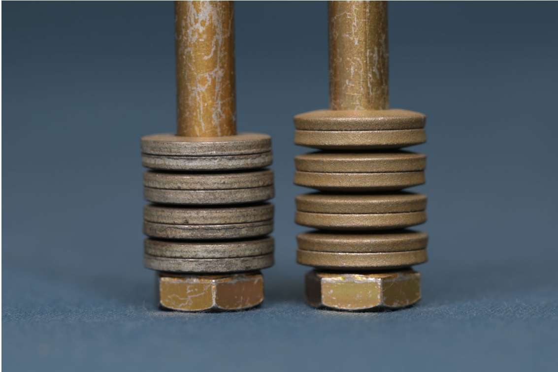
Figure 5: Comparison between a stack of occurrence (left) and exemplar (right) washers in series.
