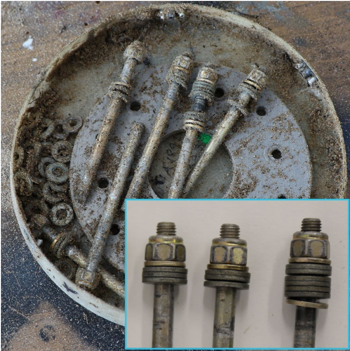
Figure 3: Propeller bolts and washers as recovered
