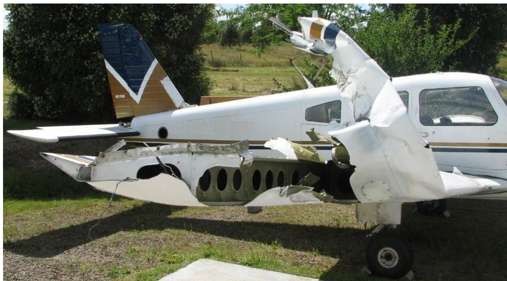
Figure 13: Damage to Piper PA-28 Warrior aircraft after mid-air collision in circuit at Coldstream Aerodrome, Vic.
