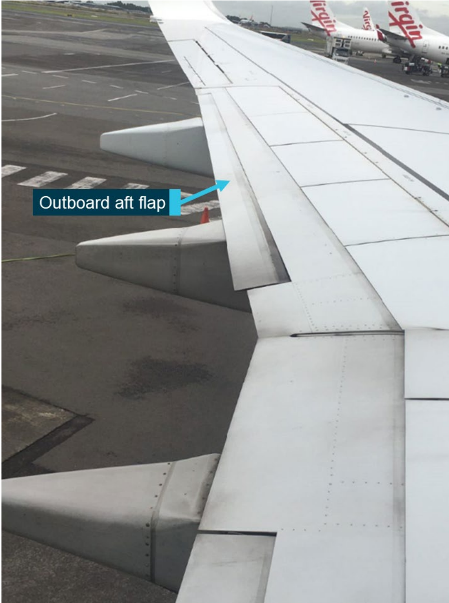
Figure 1: The skewed left outboard aft flap of VH-YFZ after landing in Sydney
