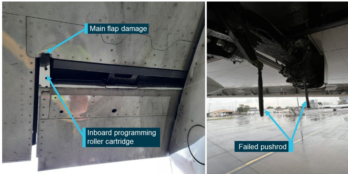
Figure 3: The programming roller cartridge obstructed by the main flap (left) and the failed pushrod (right)
