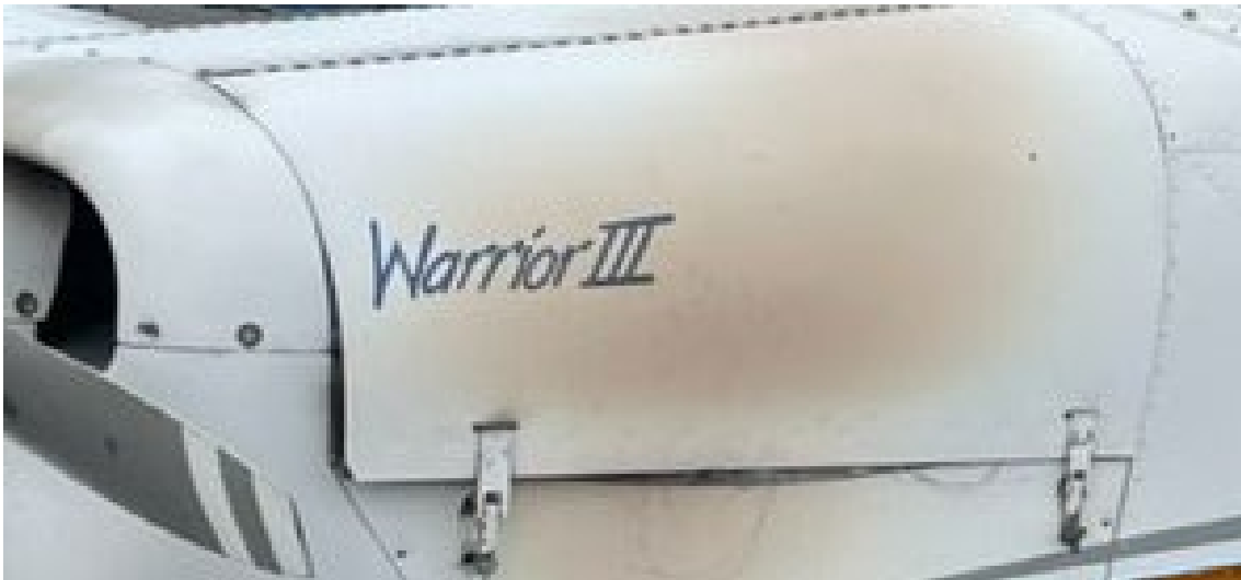
Figure 1: Burnt engine cowling
