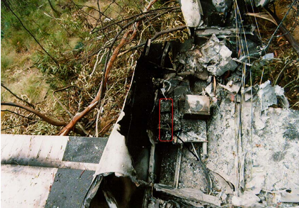
Figure 9: Wreckage of the Piper Cherokee 37 km east of Coolah, NSW (the location of the burnt ELT is outlined in red)
