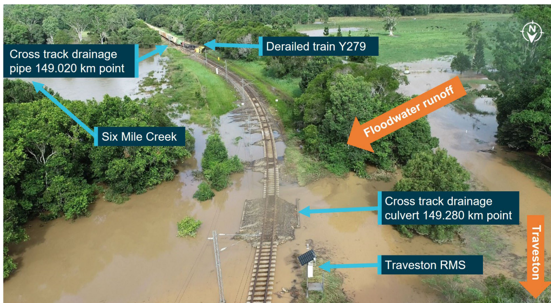
The image taken later the day of the derailment shows the relative locations of the derailed train Y279, cross track drains and the Traveston RMS. Source: ATSB
