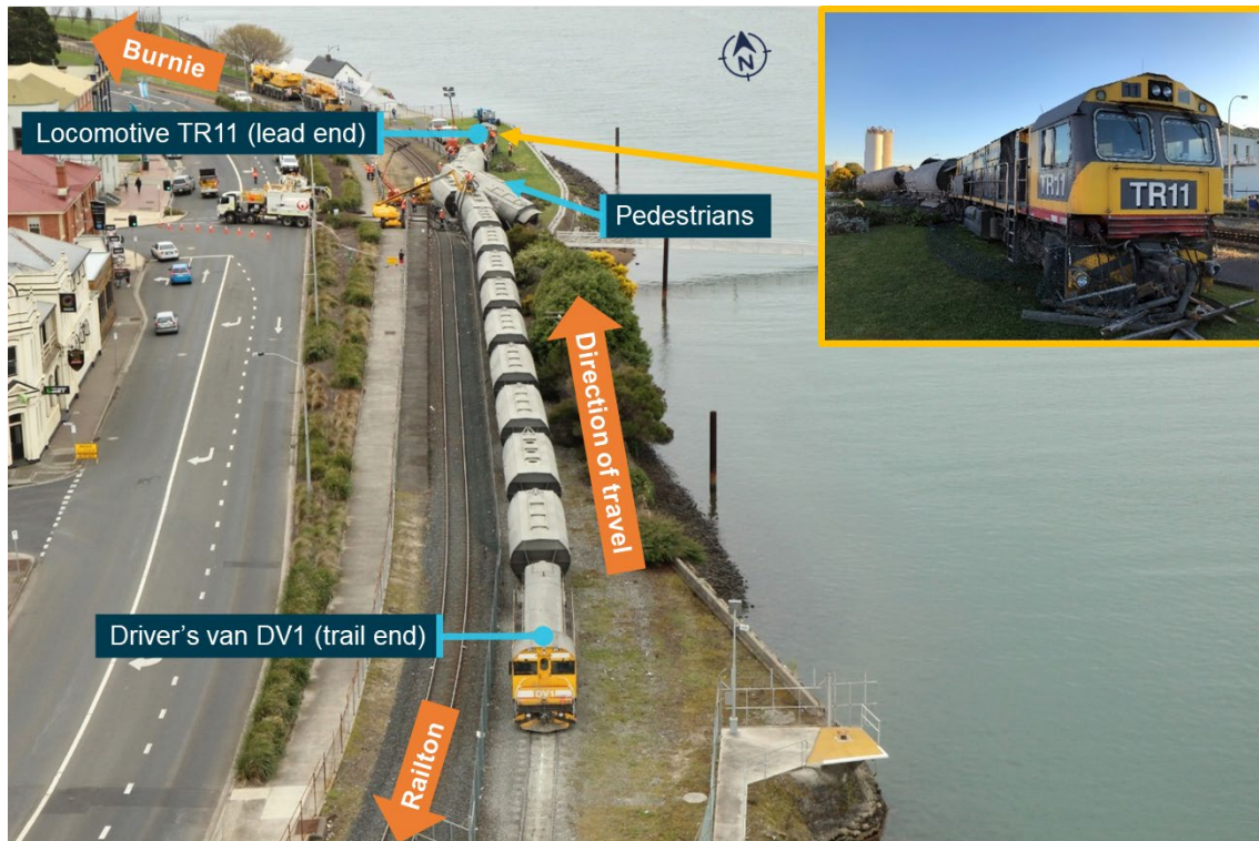
Image shows the location of the injured pedestrians at the time of the derailment, as well as the cement train consist configuration. Source: ATSB
