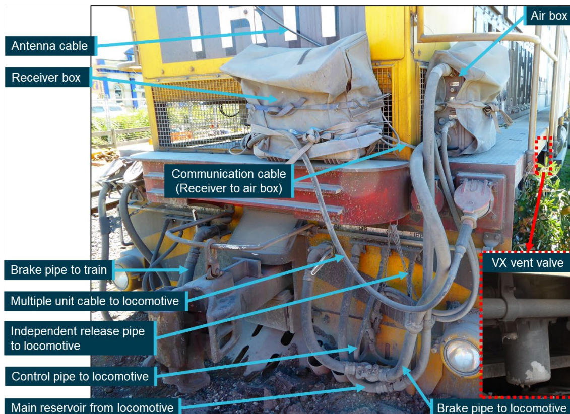
Figure 11: Rear of TR class locomotive, showing interface with generation 3 RCE
