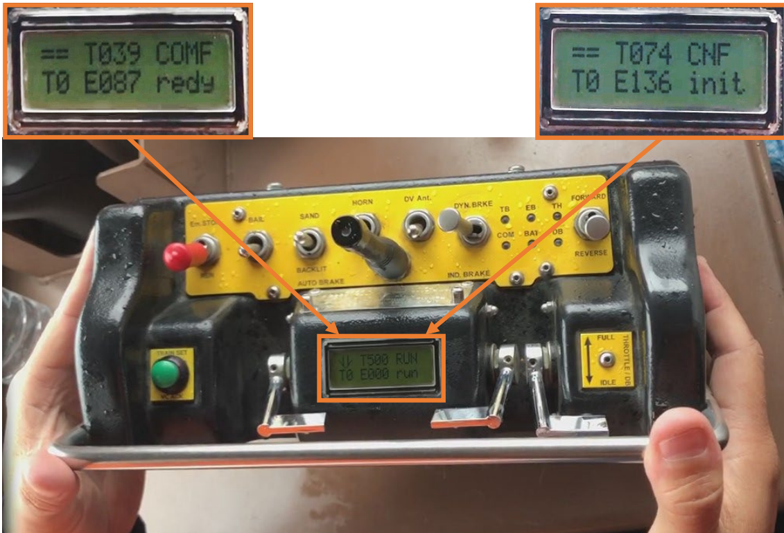
Image shows the RCE transmitter with detail images of communication failed mode (left) and control fault mode (right) presentations on the transmitter screen. Source: ATSB
