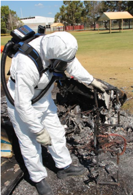
Figure 9: Investigator wearing appropriate protective equipment in response to the carbon fibre risk at the site of a Glassair III aircraft accident near Jandakot, Western Australia, on 9 December 2013
