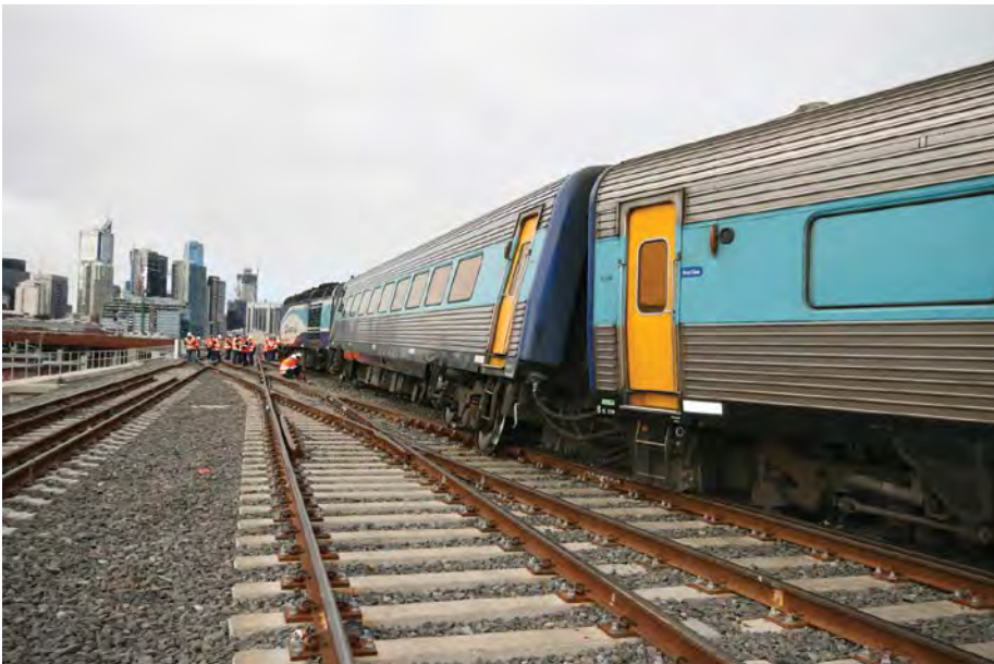
Figure 10: Derailed carriage XAM2176 Source: CITS.
