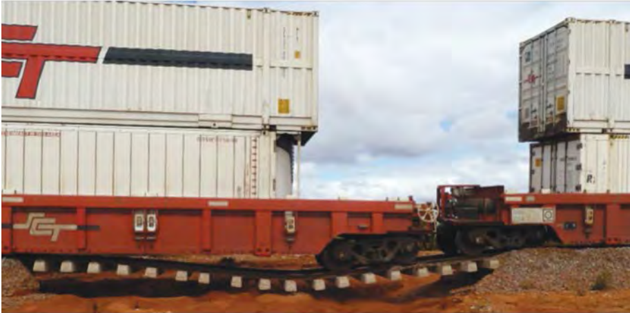
Figure 12: Well wagons on skeletal track near point of derailment. Source: ATSB.
