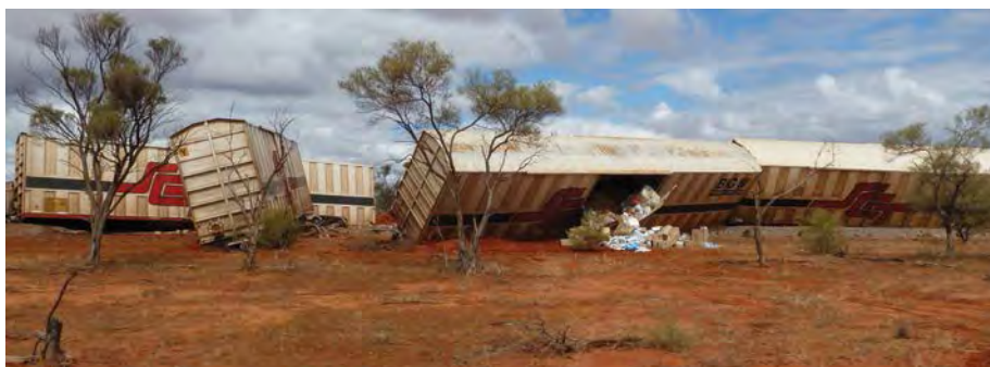
Figure 11: Derailed wagon on the north side of the track. Source: ATSB.
