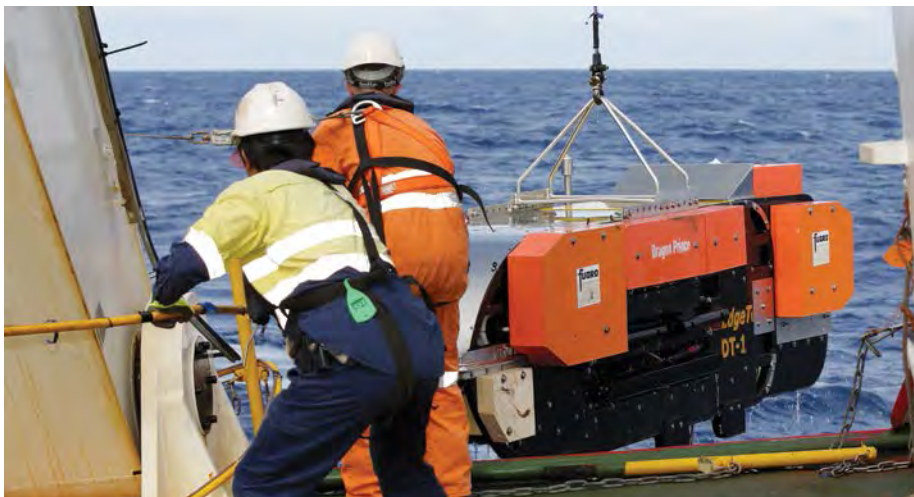
Figure 2: The Dragon Prince deep towfish is recovered onto the back deck as Fugro Discovery completes the first stage of the search for MH370. Source: ATSB, photo by ABIS Chris Beerens, RAN.
