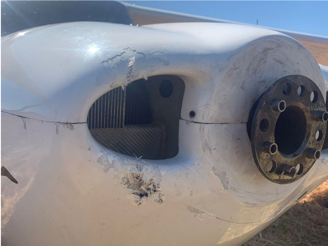
Figure 1: Propeller flange and nose cowl damage
