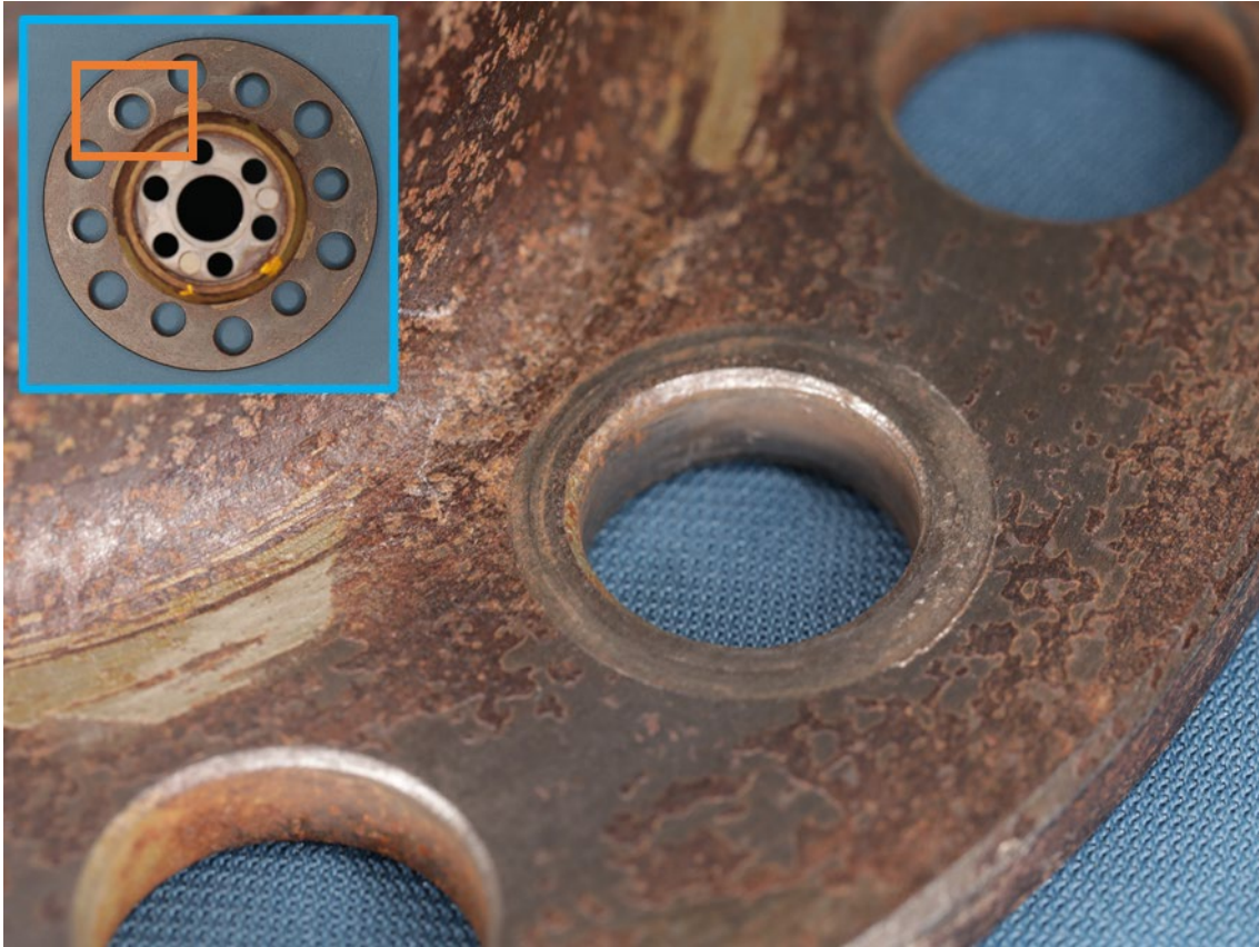
Figure 4: Wear from drive bush on propeller flange
