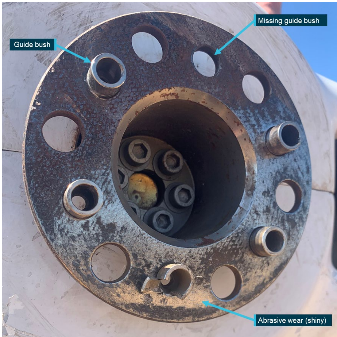
Figure 3: Propeller flange detail
