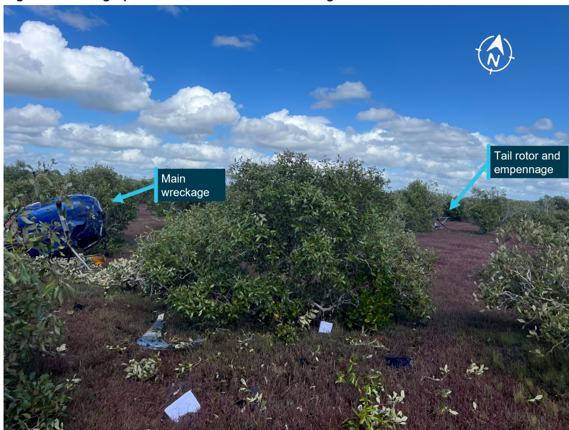
Figure 5: Photograph of main and tail rotor wreckage at accident site
